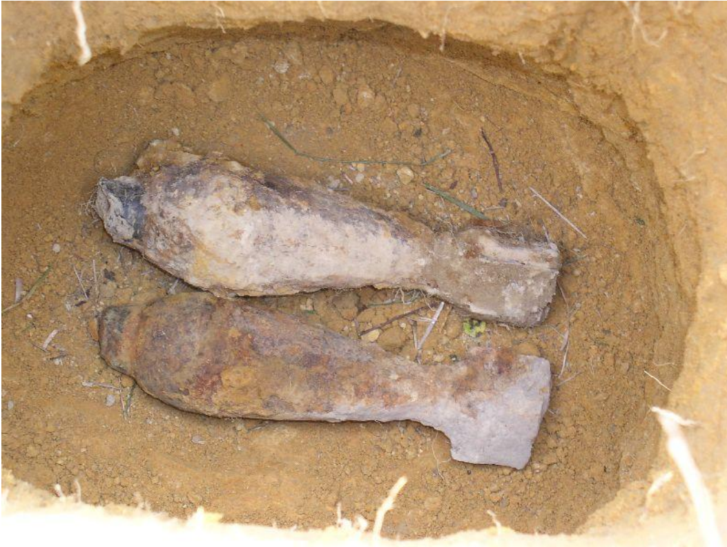
Figure C-15: Placement of two 81mm mortars in blowhole for demolition
