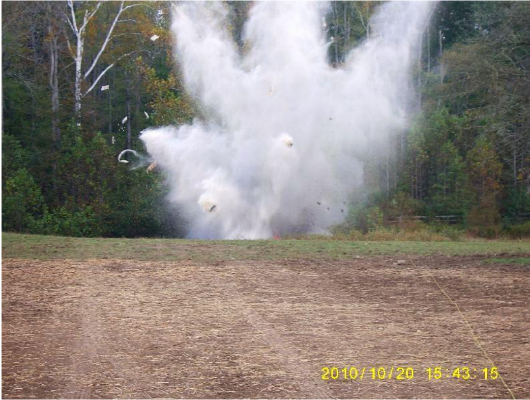
Figure C-25: Demolition clean-up shot of 155mm projectile
